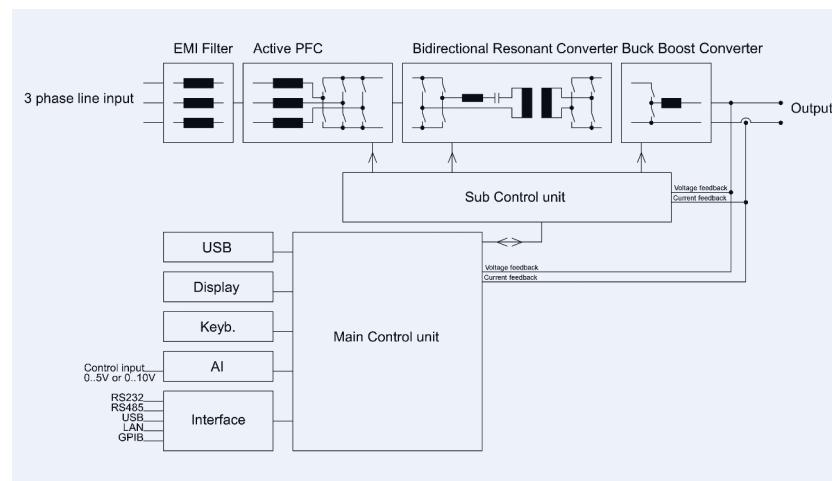
*The output of the PFC is followed by a DC/DC converter, which is also bidirectional. This takes over the galvanic isolation and has an output voltage of about 1000V. As the converter works with a almost constant output voltage, it is able to executed in full resonance. This is why it achieves a very good efficiency.*
